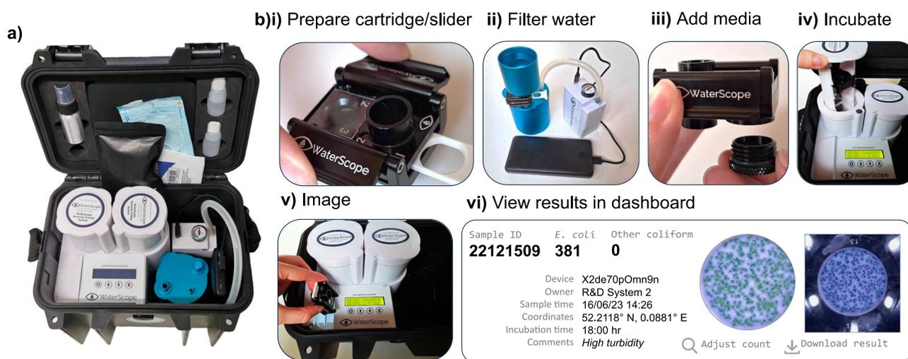
**Fig. 1 | Overview of the WaterScope test kit. a** Key components shown packed inside the system's case, weighing 6 kg with a size of 29 cm × 23 cm × 26 cm. **b** Key steps required for a single *E. coli* test. Note that a single power bank provides
