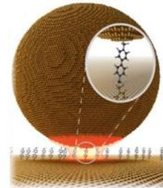
Plasmonic nanoreactors: Our group is leveraging their knowledge of nanoscale plasmonics to develop new self-assembled plasmonics nanoreactors. These utilize the million field enhancements, obtained in tight plasmonic nanogaps, to enhance photocatalytical processes. The aim of this project is to develop efficient optically driven and scalable nanotechnologies for converting otherwise resistant materials such as plastics, biowaste and CO<sub>2</sub>.
