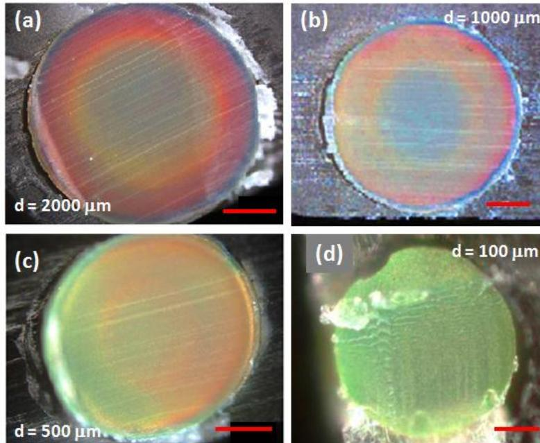
Fig. 3. Dark-field microscopy images of transverse cross-sections of red-opal fibers, showing concentric substructure. The fiber diameters,  $d$ , are as indicated; the scale bars have lengths of (a) 500  $\mu\text{m}$ , (b) 250  $\mu\text{m}$ , (c) 200  $\mu\text{m}$  and (d) 25  $\mu\text{m}$ .
