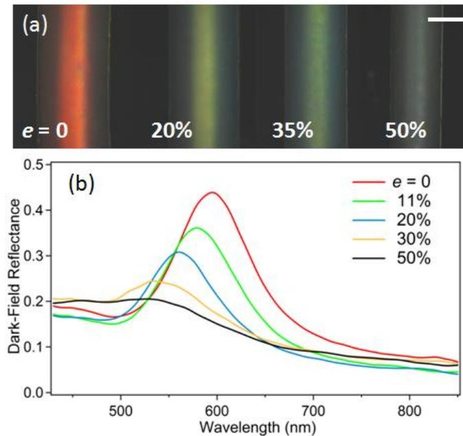
Fig. 2. (a) Dark-field  $\times 5$  images of  $1000\ \mu\text{m}$  diameter red-opal fiber at strains (left to right, in montage) of  $e = 0$ , 20%, 35% and 50%. The scale bar is  $500\ \mu\text{m}$  long. (b) Corresponding dark-field reflectance spectra for different strains.
