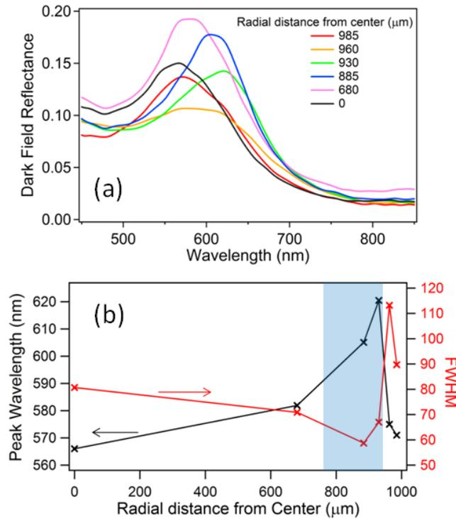
Fig. 4. (a) Dark-field reflectance spectra collected at increasing radial positions on the fiber transverse cross-section shown in Fig. 3(a) (radius = 1000  $\mu\text{m}$ ). (b) Peak wavelength and spectral FWHM of spectra as a function of radial distance from the fiber centre. The blue-shaded region indicates the zone of best ordering, where the FWHM < 70 nm
