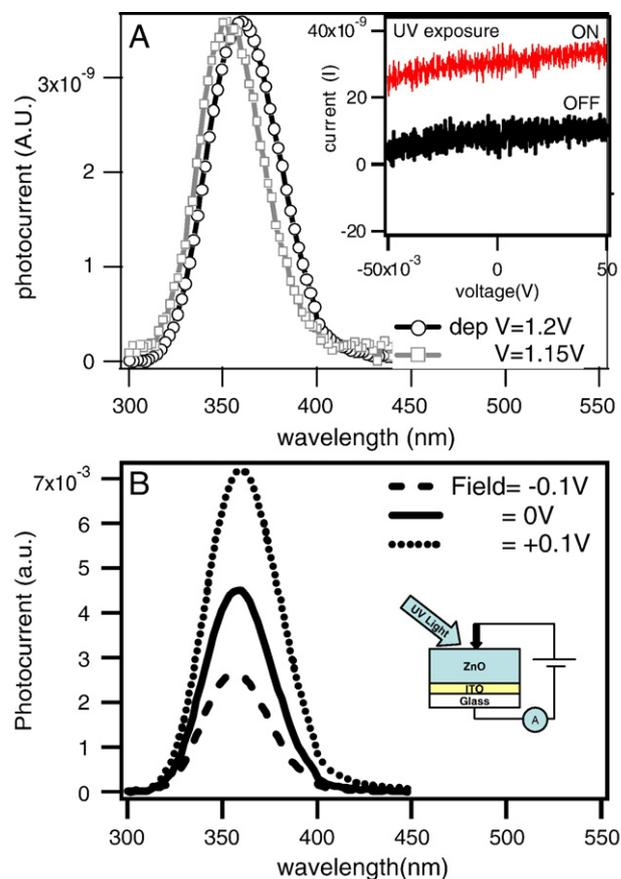
Fig. 4. (A) Photocurrent vs incident light wavelength (bias voltage= $-0.1$  V) for ZnO thin films, fabricated from different deposition potentials  $1.2$  V and  $1.15$  V. (Inset is forward I–V characteristics for UV light ON and OFF); (B) Photocurrent vs incident light wavelength for ZnO thin film (deposited at  $-1.2$  V) under various bias voltages.
