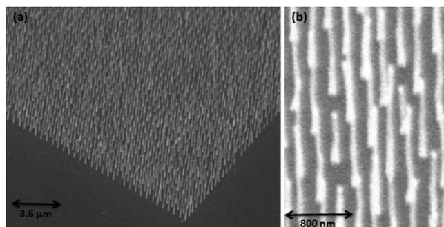
FIG. 2. (a) Electron microscopy image of a 2D square lattice array of MWCNTs having radius of 50 nm and lattice constant of 400 nm, grown on silicon substrate using PECVD. (b) The same in higher resolution.
